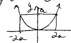
①  $\Rightarrow \text{So } dV = \frac{2}{3} y^2 \Delta x$  (Area of parabola  $\times$  thickness)
